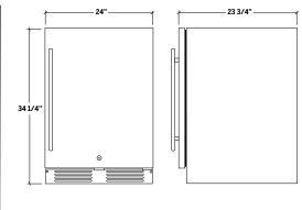
PRODUCT HR-RUO-24-1 Capacity (L) 162 L 34-50°F/1-10°C Temperature range Overall dimensions 24" x 34 1/4" x 23 3/4" (WxHxD)
